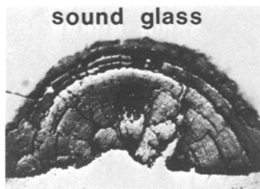
Figure 3 Optical micrograph showing biological corrosion on the glass of Evron (seen edge-on \times 160 ).
